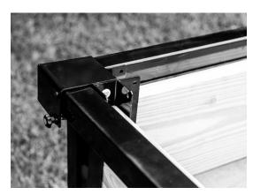
NOTE: Ensure the welded "Anti-Kick Back" tab is properly pushed up against the front side of the trailer's upright post to guarantee proper length. (See image in Step 7)
